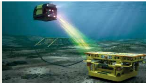
Getting a UUV to within five to ten metres of a subsea charging station is a solved problem; guiding it to docking precision without GPS remains a challenge (© Unplugged)
