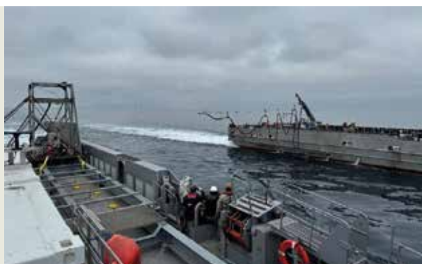
In a test as part of the NOMARS programme, the USV Mariner (right) deploys a refueling probe towards the USV Ranger (left) in the first test of fueling at sea (FAS) without any human interaction required on the part of the receiving vessel. The personnel aboard the Ranger are observers only (© DARPA)
