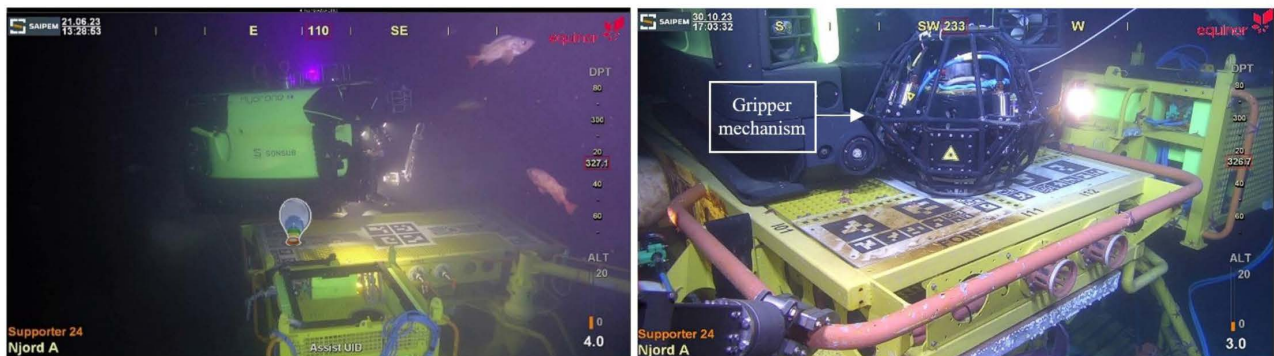
Figure 16—(left) Hydrone R approaching the SDS, guided by magnetic fields emitted by the 2.5 kW inductive coupler; (right) Hydrone R securely docked to the SDS, with the gripper mechanism anchoring the drone to the 2.5 kW inductive primary coupler
