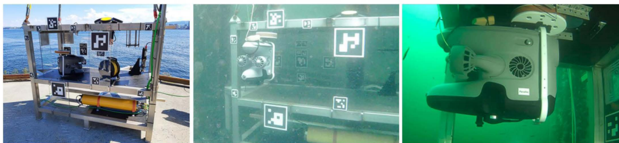
Figure 19—Docking station equipped with fiducial markers and funnel charging. The vehicle performs autonomous docking manoeuvres from Moslåttn.
