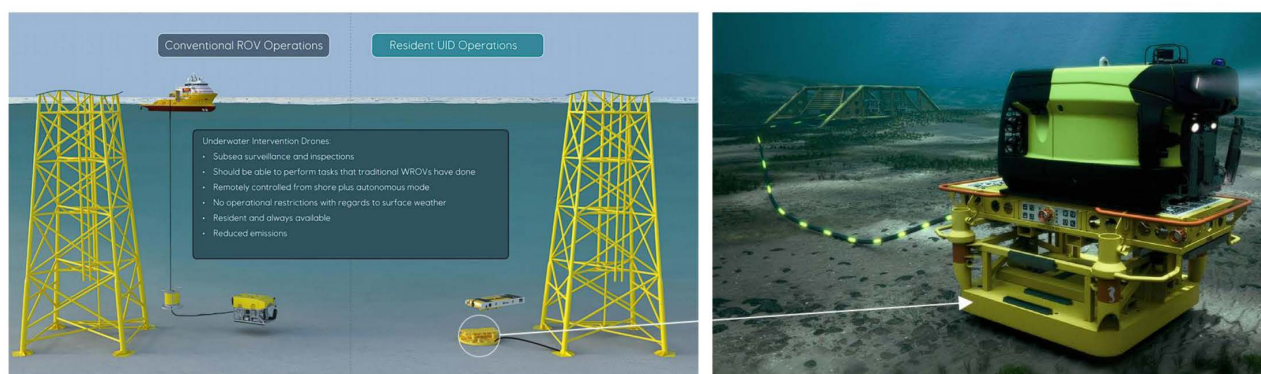
Figure 1—(left) Traditional ROV operation compared to resident UID operation, (right) SDS concept visualisation, a docked UID recharging and transferring data.
