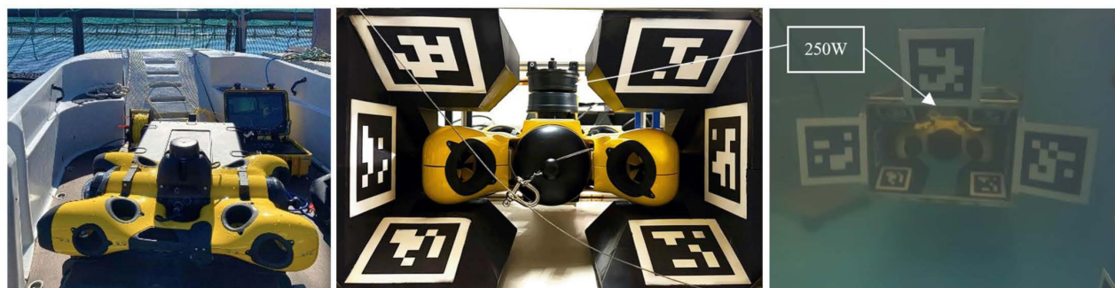
Figure 20—Hydromea charging station concept for the EXRAY using the same inductive technology used in Sudmann, 2023 and Moslåttn (2024).
