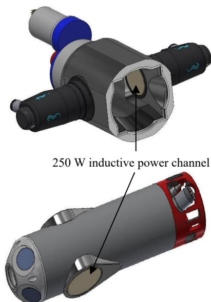
Fig. 7. Wireless charging configuration
