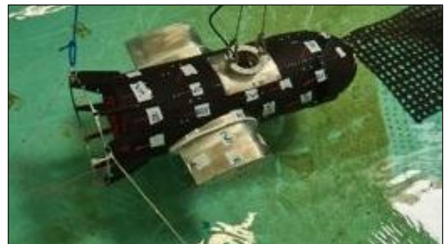
Fig. 5. The towhead structure under swimming pool tests
