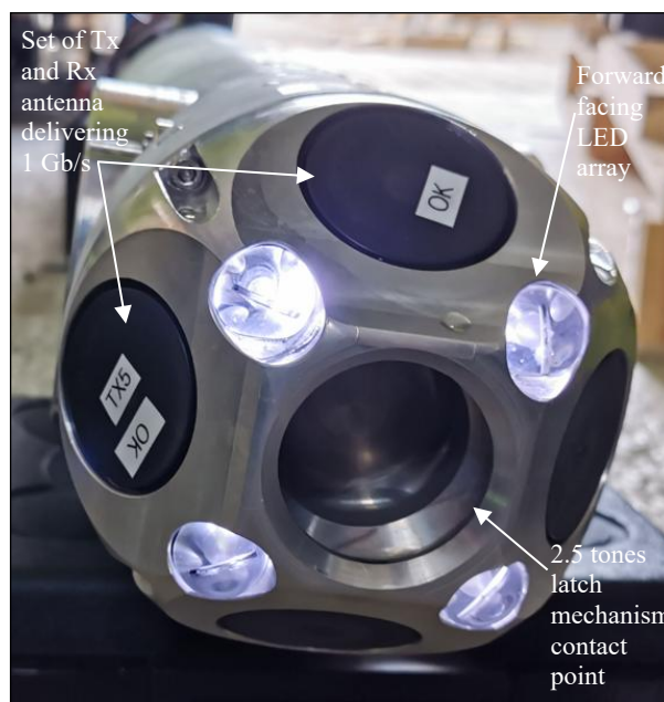
Fig. 8. Front view of the modified AUV showing the wireless gigabit antennas
