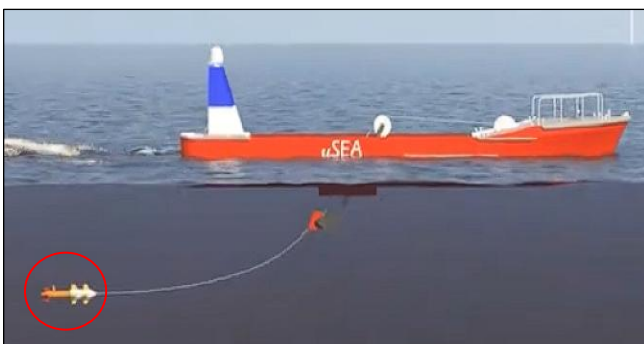
Fig. 1. USV-Towed Submerged Docking Station for AUV Recharge and Rapid Data Offload
