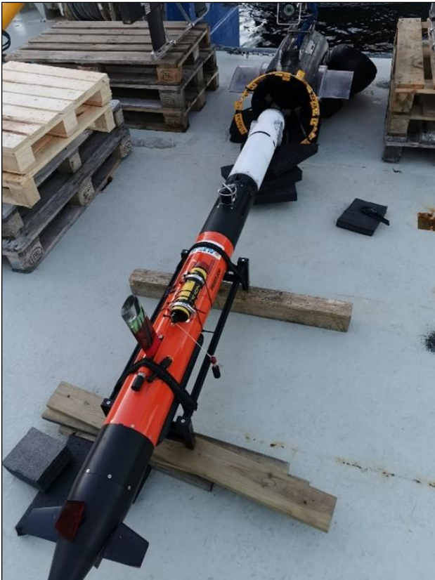
Fig. 9. AUV and towhead docking station tested in Åsenfjorden, Trondheim Fjord (Norway). Extended-duration tests performed on wet deck showed that the inductive couplers supported reliable charging, mission preparation, and high-speed data transfer eliminating the need for temporary deck cables and simplifying pre-deployment workflow
